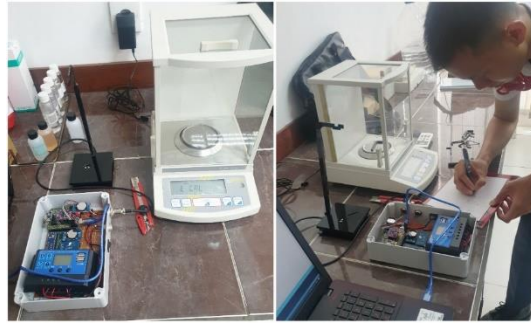
Gambar 17. Proses kalibrasi sensor Load Cell
